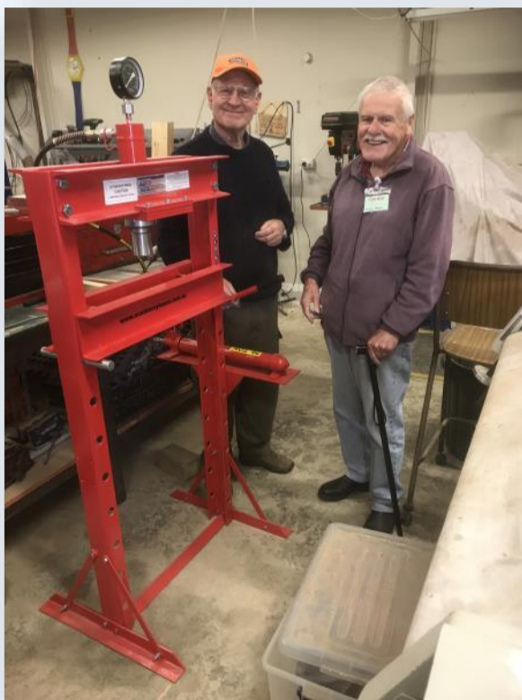
The metal men, Trevor and Gordon admiring our new toy...a 20 ton hydraulic press. This will come in handy for pressing out bearings and all other tasks the press is designed to do and is part of our metalwork arsenal.
