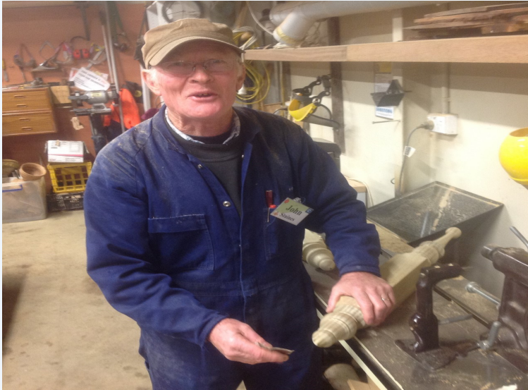
John Staines has done a good job of making a replica turned finial from a weathered one to a new one which will last another 20 years when properly painted.
