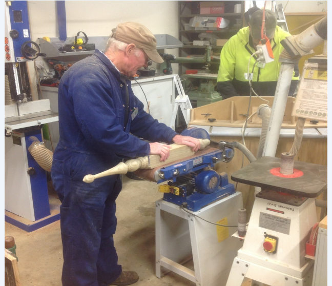
John Staines has done a good job of making a replica turned finial from a weathered one to a new one which will last another 20 years when properly painted.
